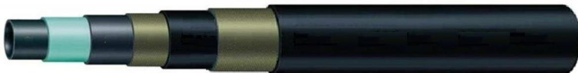
Tube- CR Barrier - PA Friction-NBR Reinforcement - PET Friction-NBR Reinforcement - PET Cover - EPDM
